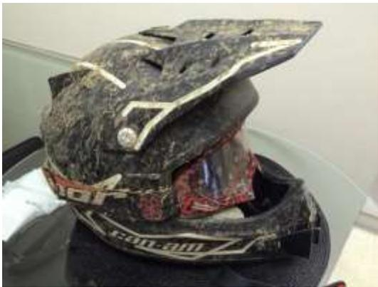
“A helmet is only good for one impact,” says Meed. “If you dent or crack your helmet, you must get a replacement helmet right away. Helmets are made in such a fashion that a blow will impact their integrity, even if it is not apparent while viewing.”
